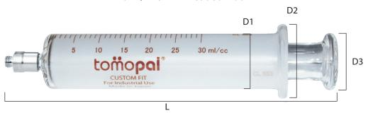
Tomopal Part #140-7030Piston Outside Diameter:22.90 mm ± 0.20 mmD1) Barrel Diameter Outside:27.30 mm ± 0.40 mmD2) Barrel Collar Diameter:37.55 mm ± 0.75 mmD3) Piston Collar Diameter:27.95 mm ± 0.65 mmL) Length:164.00 mm ± 0.50 mmIncrement:1.0 ml
